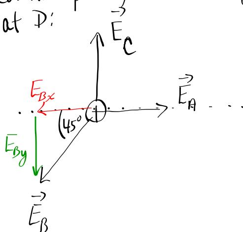
$$|\vec{E}_A| = \frac{kQ_A}{r_A^2} = \frac{k(6.0 \times 10^{-6} C)}{(0.050 m)^2} = 2.16 \times 10^7 N/C$$
