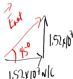
$$\vec{E}_{\text{net}} \text{ at } D = 2.15 \times 10^7 N/C$$
